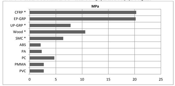
Average lap shear strengths of typical non-metallic substrates joints (ISO 4587) (typical average values)
